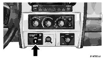
**NOTE:** The Passenger Airbag On/Off Switch is not available in the Ouad Cab.
